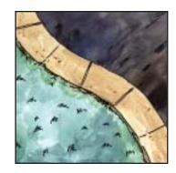
Place SplitStone edging along the established alignment, and on top of the fabric or plastic.
