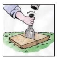
6. To cut SplitStone to match the desired length at the end of your project, simply score a line across the edger with a chisel and hammer. A saw with a masonry blade may also be used. Always wear eye protection.
